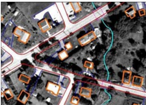
Digital Vector Mapping of Geographic Features (e.g., Roads, Buildings, Hydrography, Structures, etc.)
