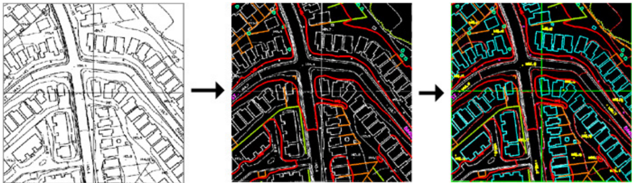
Conversion of scanned Ontario Basic Maps and Property Boundaries to GIS format.
